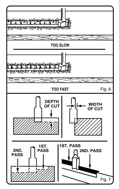
large enough cutter may not be broken off, but if the cut is too deep a rough cut will result — and it may be very difficult to guide and control the cutter as desired. For these reasons, we recommend that you do not exceed 1/8 in. (3.2 mm) depth of cut in a single pass, regardless of the cutter size or the softness or condition of the workpiece. This will result in a higher quality cut.
